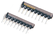
RESISTOR NETWORK Single in Line Package
