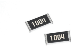
High Power < 1 ohm Thick Film
