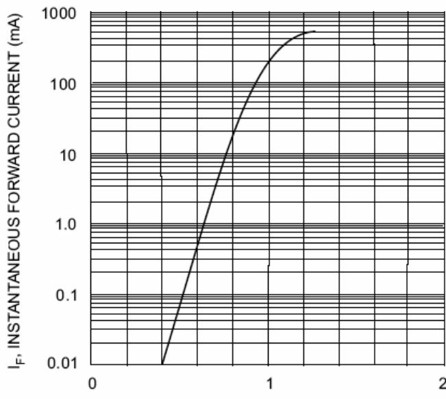
Fig. 1 Forward Characteristics
