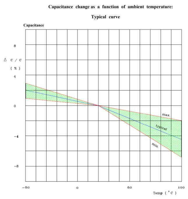
\*\* All capacitance values are specified at 1K Hz
