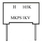
H: SYMBOL OF HITANO 103: CAPACITANCE K: TOL. MKPS: SERIES 1KV: RATED VOLTAGE
