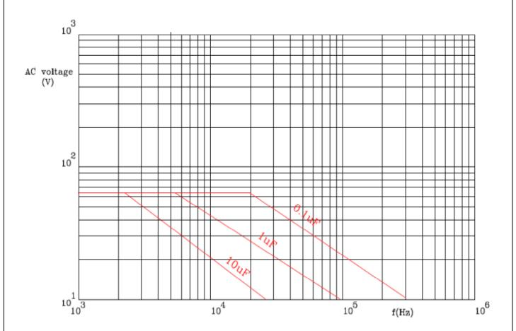
\*\* AC voltage as a function of frequency at temp≤85°C, for Vrdc=100V
