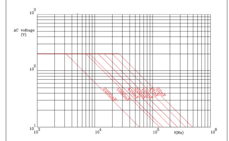
\*\* AC voltage as a function of frequency at temp≤85°C, for Vrdc=400V
