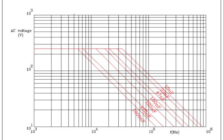
\*\* AC voltage as a function of frequency at temp≤85°C, for Vrdc=630V
