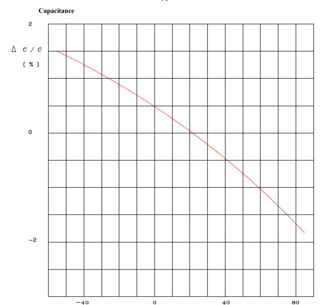
\*\* All capacitance values are specified at 1K Hz
