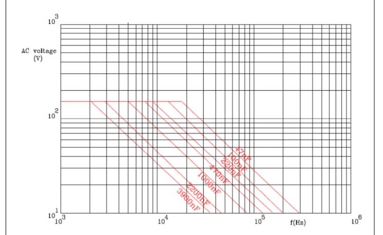
\*\* AC voltage as a function of frequency at temp  $\leq$  85°C, for Vrdc = 250V
